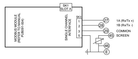
PASSIVE TERMINATION CONTRLOLED VIA SETTING IN ACTUATOR CONFIGURATION. REFER TO PUB002-040
