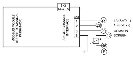
PASSIVE TERMINATION CONTROLLED VIA SETTING IN ACTUATOR CONFIGURATION. REFER TO PUB002-040
