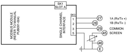
PASSIVE TERMINATION CONTROLLED VIA SETTING IN ACTUATOR CONFIGURATION. REFER TO PUB002-040
