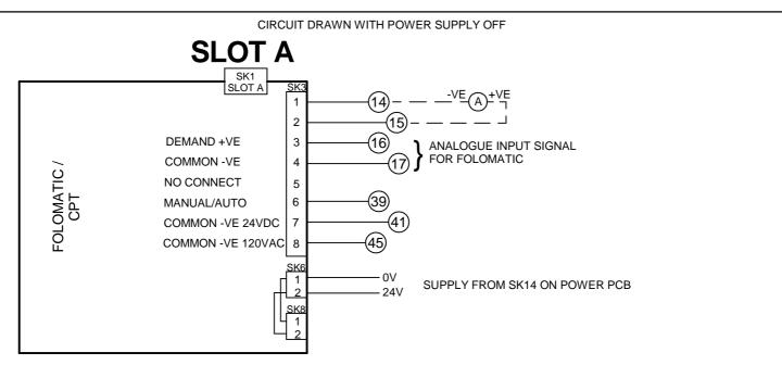
FOR MANUAL/AUTO CONNECTIONS AND DETAILS OF FOLOMATIC/CPT FUNCTIONS **REFER TO ROTORK PUBLICATION PUB002-041** FOR PAKSCAN CONTROL FOLOMATIC MUST BE CONFIGURED FOR MANUAL OPERATION
