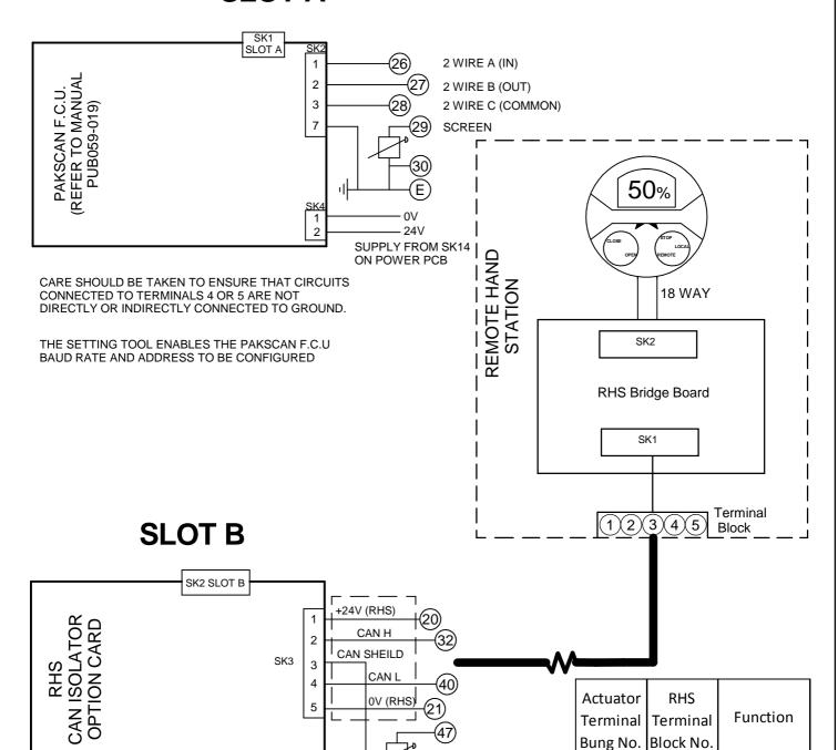
RHS CABLE IS CUSTOMER SUPPLIED, FOR SPECIFICATION SEE PUB002-059, MAXIMUM LENGTH OF CABLE TO BE 100m.
