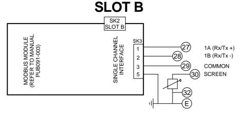
TERMINATION CONTROLLED VIA SETTING IN ACTUATOR CONFIGURATION. REFER TO PUB002-040
