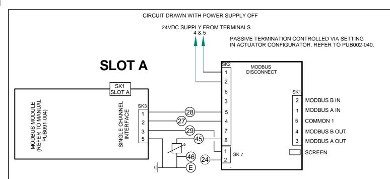
MODBUS RS485 SIGNAL LINES REQUIRE EXTERNAL ACTIVE BIASING TO BE PROVIDED AT ONE LOCATION FOR THE WHOLE BUS SEGMENT. REFER TO PUB091-004.
