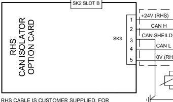
RHS CABLE IS CUSTOMER SUPPLIED, FOR SPECIFICATION SEE PUB002-059, MAXIMUM LENGTH OF CABLE TO BE 100m.
