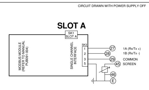
PASSIVE TERMINATION CONTROLLED VIA SETTING IN ACTUATOR CONFIGURATION. REFER TO PUB002-040
