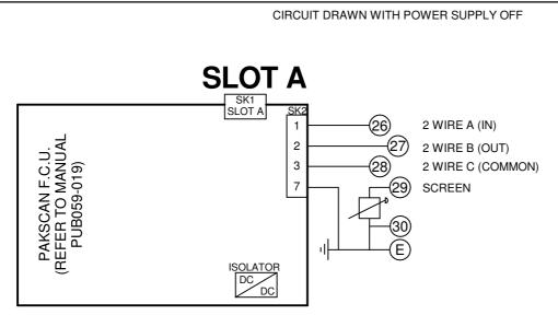
CARE SHOULD BE TAKEN TO ENSURE THAT CIRCUITS CONNECTED TO TERMINALS 4 OR 5 ARE NOT DIRECTLY OR INDIRECTLY CONNECTED TO GROUND.
