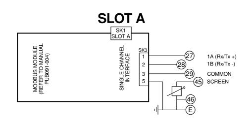
PASSIVE TERMINATION CONTROLLED VIA SETTING IN ACTUATOR CONFIGURATION. REFER TO PUB002-040
