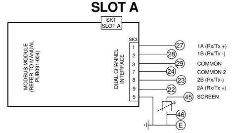
PASSIVE TERMINATION CONTROLLED VIA SETTING IN ACTUATOR CONFIGURATION. REFER TO PUB002-040
