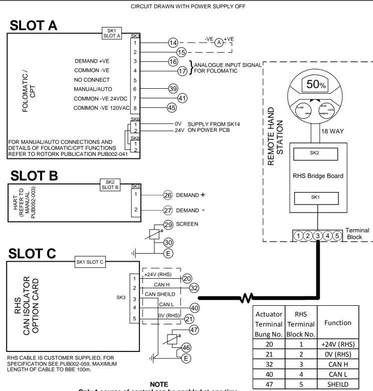
Only 1 source of control can be enabled at one time.
