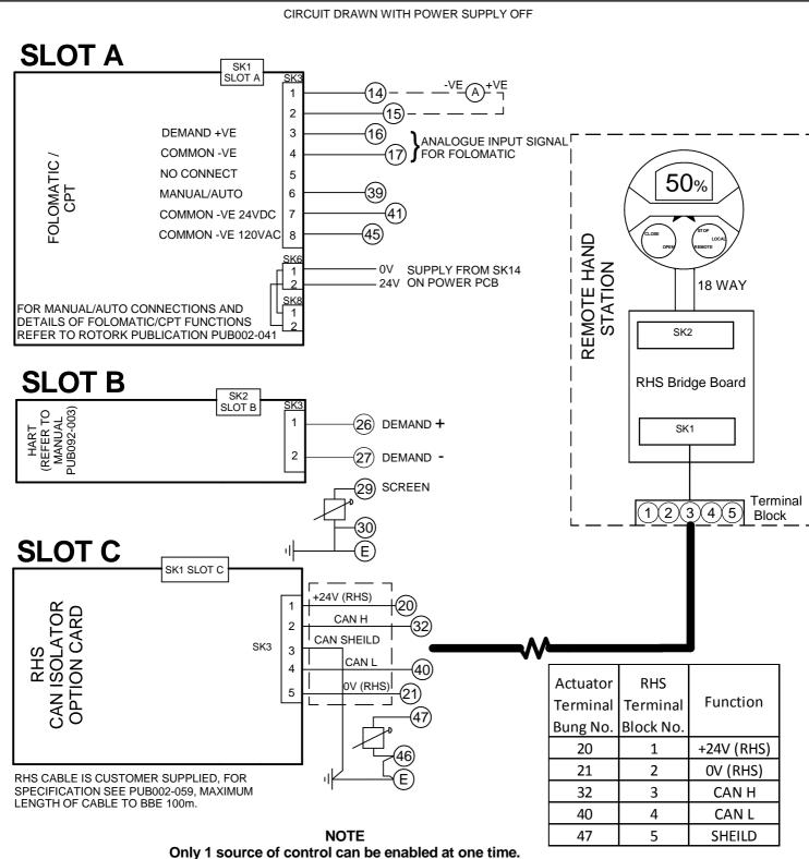
As default the folomatic will have control, selection of the other control source can be made using the manual / auto input on the folomatic card
