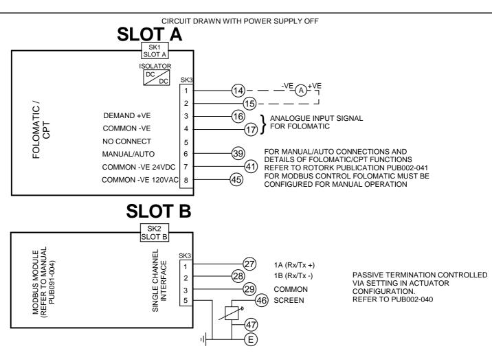
MODBUS RS485 SIGNAL LINES REQUIRE EXTERNAL ACTIVE BIASING TO BE PROVIDED AT ONE LOCATION FOR THE WHOLE BUS SEGMENT. REFER TO PUB091-004.
