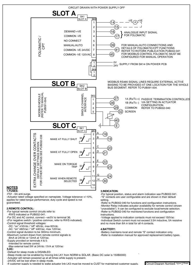
$\begin{array}{c|c} \hline \text{Circuit Diagram Number} & \begin{array}{c|c} \text{Issue} & \\ \text{No} \\ 2 & \text{of } 2 \end{array} \end{array}$
