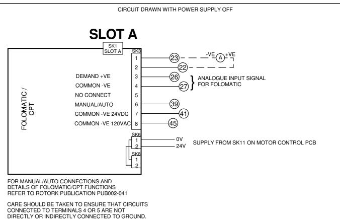
DIRECTLY ON INDIRECTLY CONNECTED TO GROUND.
