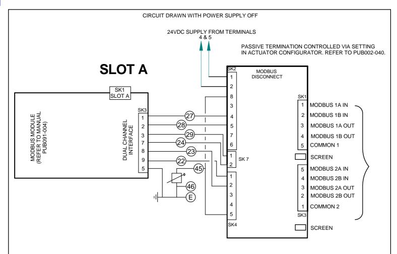
MODBUS RS485 SIGNAL LINES REQUIRE EXTERNAL ACTIVE BIASING TO BE PROVIDED AT ONE LOCATION FOR THE WHOLE BUS SEGMENT. REFER TO PUB091-004
