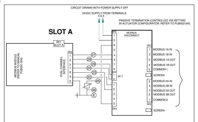
MODBUS RS485 SIGNAL LINES REQUIRE EXTERNAL ACTIVE BIASING TO BE PROVIDED AT ONE LOCATION FOR THE WHOLE BUS SEGMENT. REFER TO PUB091-004
