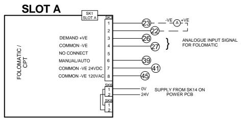
FOR MANUAL/AUTO CONNECTIONS AND DETAILS OF FOLOMATIC/CPT FUNCTIONS REFER TO ROTORK PUBLICATION PUB002-041 FOR PAKSCAN CONTROL FOLOMATIC MUST BE CONFIGURED FOR MANUAL OPERATION
