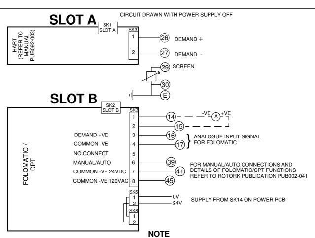
Only 1 source of control can be enabled at one time. As default the folomatic will have control, selection of the other control source can be made using the manual / auto input on the folomatic card
