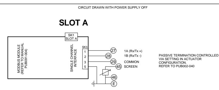
MODBUS RS485 SIGNAL LINES REQUIRE EXTERNAL ACTIVE BIASING TO BE PROVIDED AT ONE LOCATION FOR THE WHOLE BUS SEGMENT. REFER TO PUB091-004.
