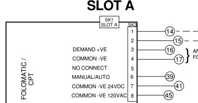
NOTE - UNDER LOSS OF AC POWER CPT OUTPUT WILL GO TO LESS THAN 1mA
