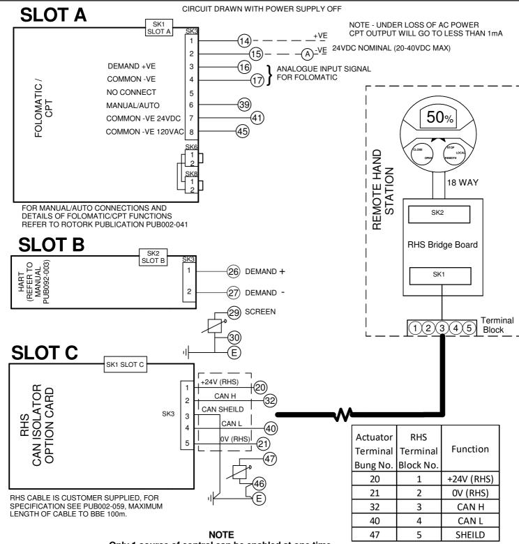
Only 1 source of control can be enabled at one time. As default the folomatic will have control, selection of the other control source can be made using the manual / auto input on the folomatic card
