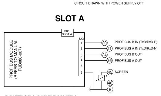
THE SETTING TOOL ENABLES THE PROFIBUS ADDRESS TO BE CONFIGURED.
