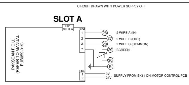
CARE SHOULD BE TAKEN TO ENSURE THAT CIRCUITS CONNECTED TO TERMINALS 4 OR 5 ARE NOT DIRECTLY OR INDIRECTLY CONNECTED TO GROUND.
