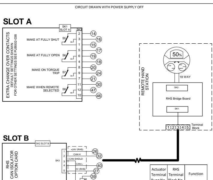
RHS CABLE IS CUSTOMER SUPPLIED, FOR SPECIFICATION SEE PUB002-059, MAXIMUM LENGTH OF CABLE TO BE 100m.
