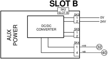
SUPPLY FROM SK11 ON MOTOR CONTROL PCB
