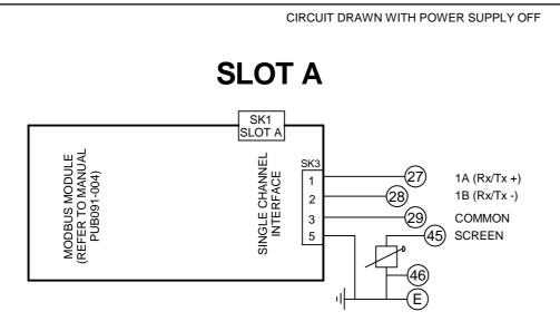
PASSIVE CONTROLLED VIA SETTING IN ACTUATOR CONFIGURATION. REFER TO PUB002-040
