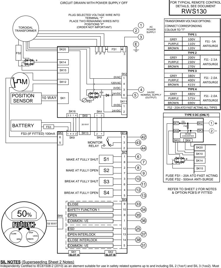
be installed, commissioned, tested and operated fully in accordance with the Safety Manual. Refer to SIL Safety Manual - PUB002-110 SIL STAYPUT (Safety Function 1): The control signal must be applied to terminal 34 before an open or closed control signal will operate the actuator. This is a high demand safety function, actuator will not move spuriously. The SIL STAYPUT function is not applicable for LOCAL control.
