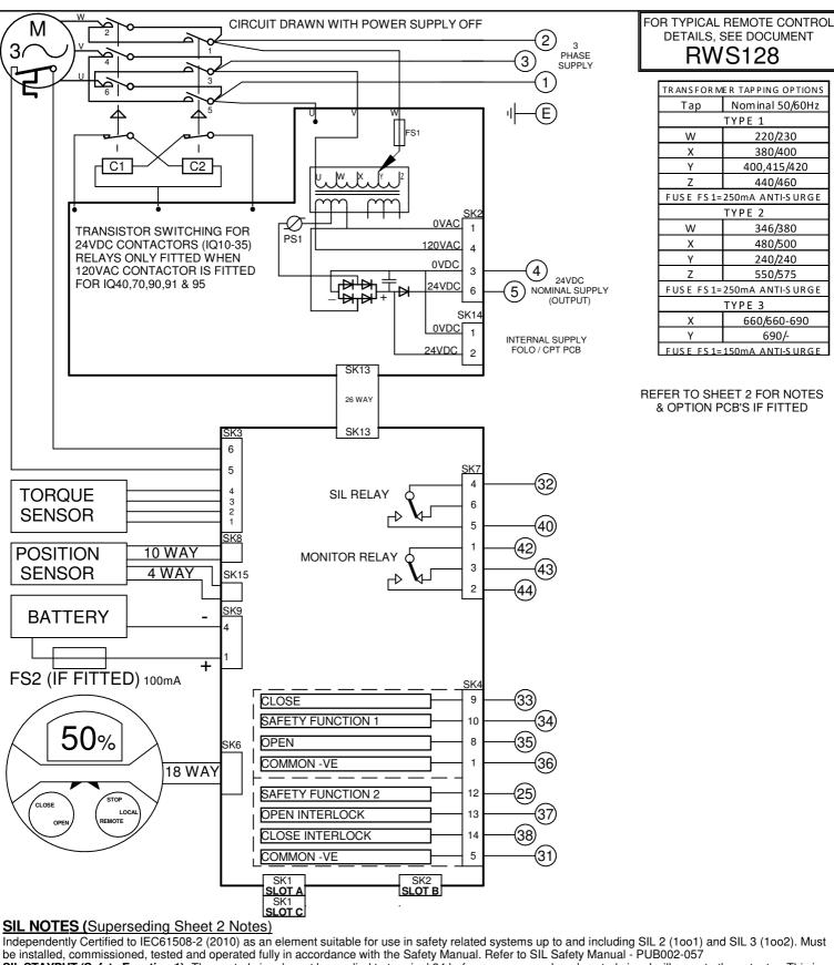
SIL STAYPUT (Safety Function 1): The control signal must be applied to terminal 34 before an open or closed control signal will operate the actuator. This is a high demand safety function, actuator will not move spuriously.
