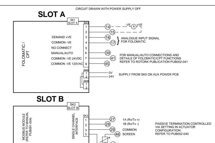
MODBUS RS485 SIGNAL LINES REQUIRE EXTERNAL ACTIVE BIASING TO BE PROVIDED AT ONE LOCATION FOR THE WHOLE BUS SEGMENT. REFER TO PUB091-004.
