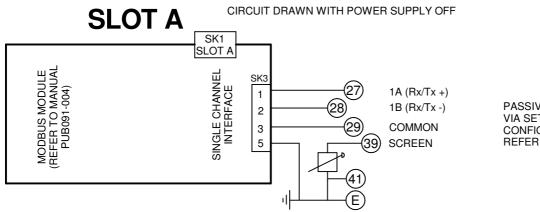
PASSIVE TERMINATION CONTROLLED VIA SETTING IN ACTUATOR CONFIGURATION. REFER TO PUB002-040
