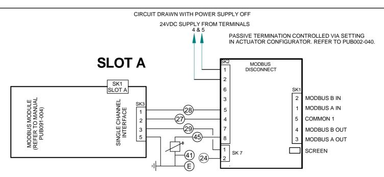
MODBUS RS485 SIGNAL LINES REQUIRE EXTERNAL ACTIVE BIASING TO BE PROVIDED AT ONE LOCATION FOR THE WHOLE BUS SEGMENT. REFER TO PUB091-004.
