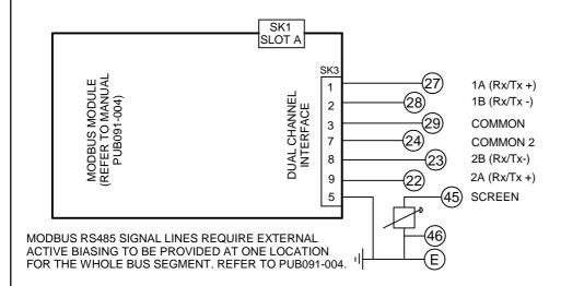
PASSIVE TERMINATION CONTROLLED VIA SETTING IN ACTUATOR CONFIGURATION. REFER TO PUB002-040
