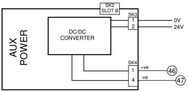
SUPPLY FROM SK11 ON MOTOR CONTROL PCB
