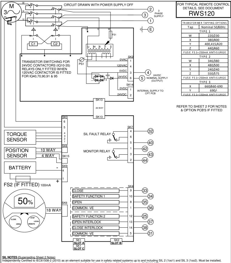
commissioned, tested and operated fully in accordance with the Safety Manual. Refer to SIL Safety Manual - PUB002-057 SIL STAYPUT (Safety Function 1): The control signal must be applied to terminal 34 before an open or closed control signal will operate the actuator. This is a high demand safety function, actuator will not move spuriously.
