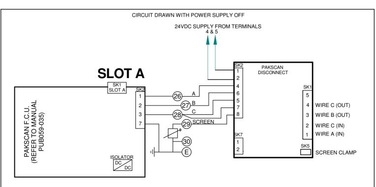
CARE SHOULD BE TAKEN TO ENSURE THAT CIRCUITS CONNECTED TO TERMINALS 4 OR 5 ARE NOT DIRECTLY OR INDIRECTLY CONNECTED TO GROUND.
