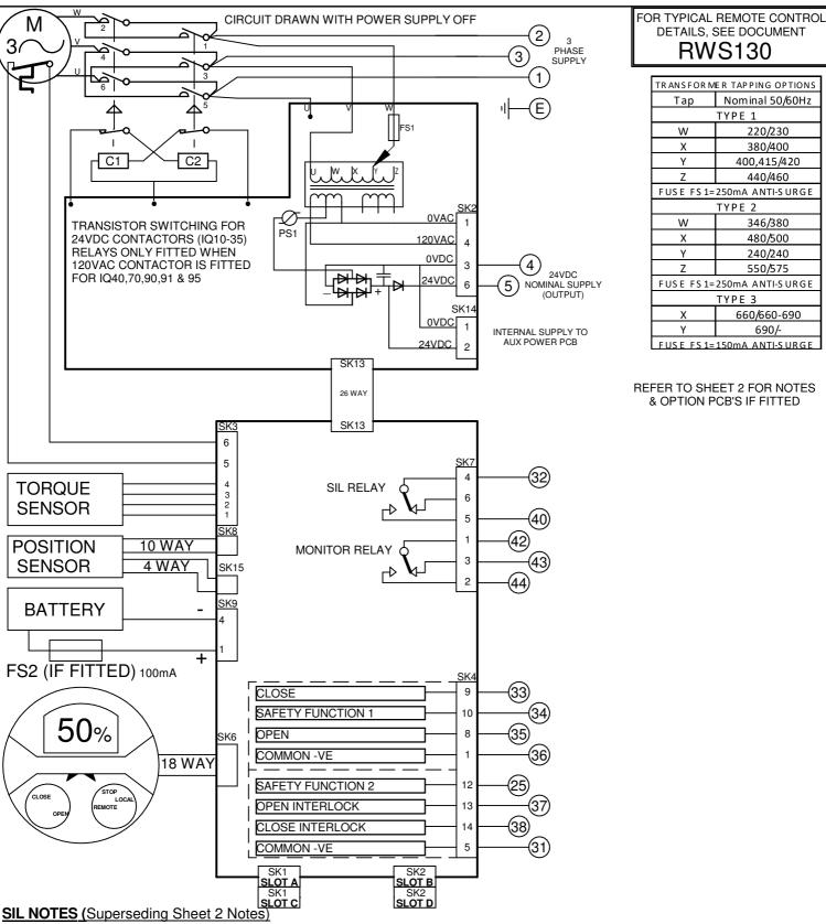
Independently Certified to IEC61508-2 (2010) as an element suitable for use in safety related systems up to and including SIL 2 (1001) and SIL 3 (1002). Must be installed, commissioned, tested and operated fully in accordance with the Safety Manual. Refer to SIL Safety Manual - PUB002-057
