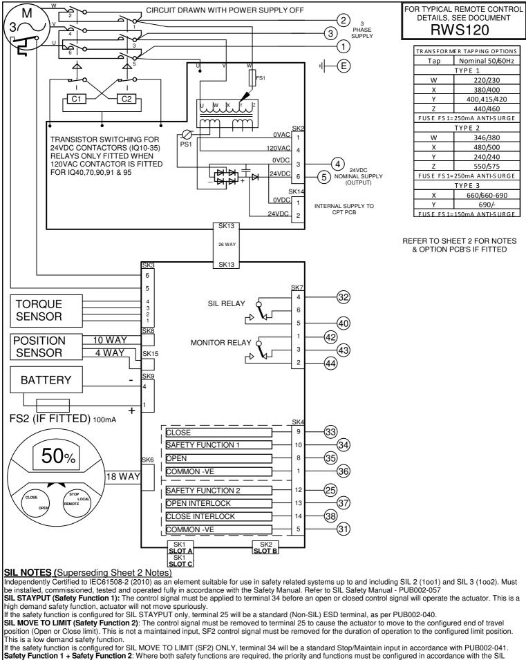
Safety Manual - PUB002-057. The common for SF1 (terminal 36) and SF2 (terminal 31) are independent allowing the control signal to be derived from separate, independent systems. If required, where signals are derived from the same system, the commons can be linked together.
