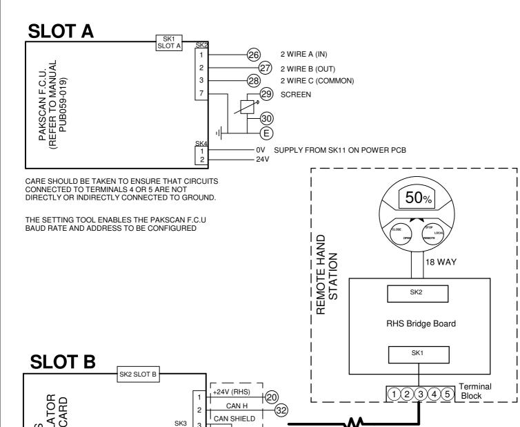
RHS CABLE IS CUSTOMER SUPPLIED. FOR SPECIFICATION SEE PUB002-059. MAXIMUM LENGTH OF CABLE TO BE 100M.
