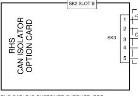
RHS CABLE IS CUSTOMER SUPPLIED, FOR SPECIFICATION SEE PUB002-059, MAXIMUM LENGTH OF CABLE TO BE 100m.
