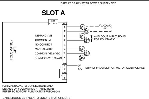
CONNECTED TO TERMINALS 4 OR 5 ARE NOT DIRECTLY OR INDIRECTLY CONNECTED TO GROUND.
