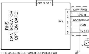
RHS CABLE IS CUSTOMER SUPPLIED, FOR SPECIFICATION SEE PUB002-059, MAXIMUM LENGTH OF CABLE TO BBE 100m.
