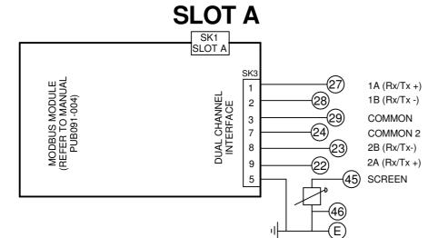
PASSIVE TERMINATION CONTROLLED VIA SETTING IN ACTUATOR CONFIGURATION. REFER TO PUB002-040
