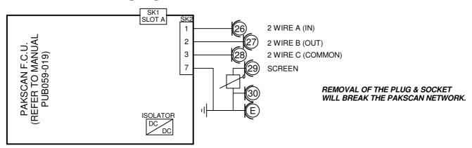
CARE SHOULD BE TAKEN TO ENSURE THAT CIRCUITS CONNECTED TO TERMINALS 4 OR 5 ARE NOT DIRECTLY OR INDIRECTLY CONNECTED TO GROUND.
