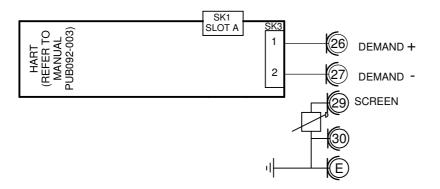
REMOVAL OF THE PLUG & SOCKET WILL BREAK THE HART NETWORK.
