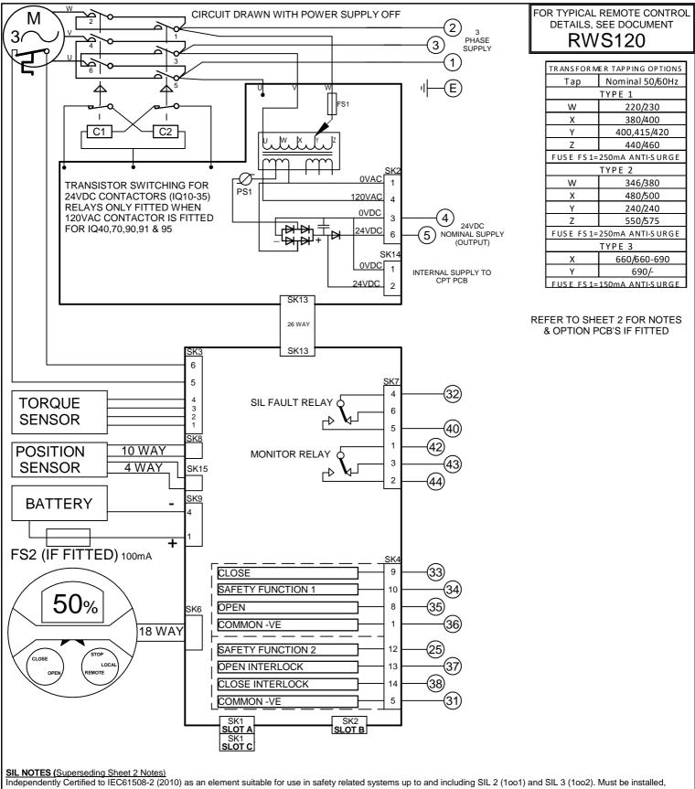
Independently Certified to IEC61508-2 (2010) as an element suitable for use in safety related systems up to and including SIL 2 (1001) and SIL 3 (1002). Must be installed, commissioned, tested and operated fully in accordance with the Safety Manual. Refer to SIL Safety Manual - PUB002-057 SIL STAYPUT (Safety Function 1): The control signal must be applied to terminal 34 before an open or closed control signal will operate the actuator. This is a high demand
