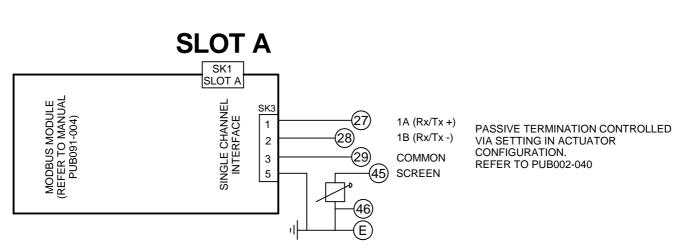
MODBUS RS485 SIGNAL LINES REQUIRE EXTERNAL ACTIVE BIASING TO BE PROVIDED AT ONE LOCATION FOR THE WHOLE BUS SEGMENT. REFER TO PUB091-004.
