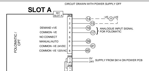
FOR MANUAL/AUTO CONNECTIONS AND DETAILS OF FOLOMATIC/CPT FUNCTIONS REFER TO ROTORK PUBLICATION PUB002-041 FOR MODBUS CONTROL FOLOMATIC MUST BE CONFIGURED FOR MANUAL OPERATION
